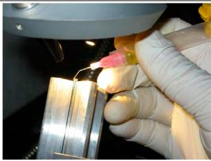
Example of front element assembly on a laparoscope diameter 7mm
