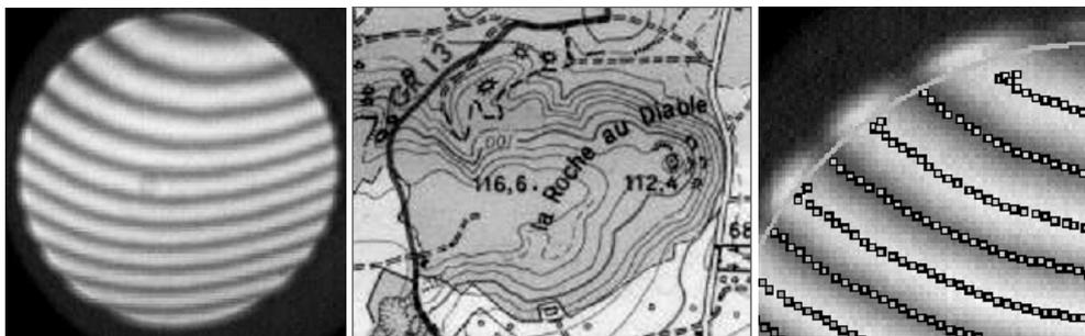
Fig. 1 The fringes peaks and valleys are level curves of the wavefront.
